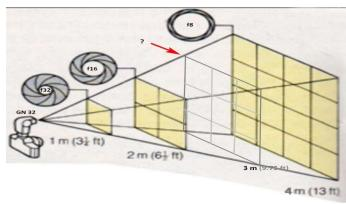
If you intensify the light beam by narrowing it with a lens or reflector the Guide Number goes up. If you reduce the power output of the flash you reduce the Guide Number
