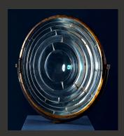
Fresnell lights (note the odd spelling, fre-nell from the French inventor) have concentric rings formed into the lens. Each ring bends the light more until it converges into a single beam of light.
