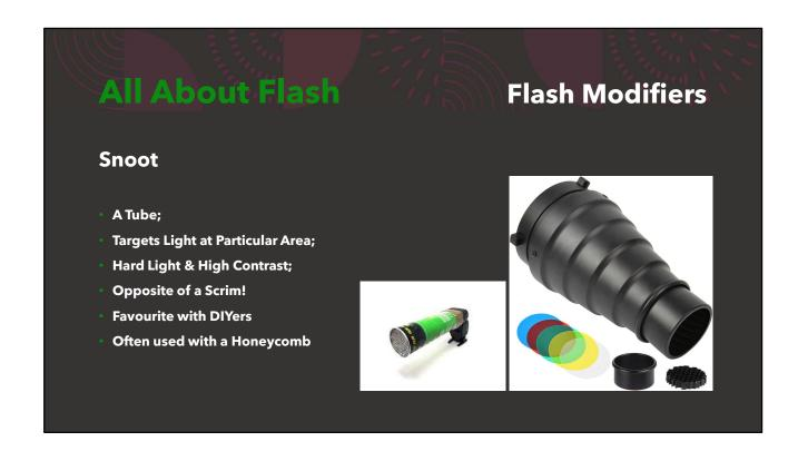
A snoot is a tube that goes over the front of the light, acting as a spotlight and allowing one to light the main subject without the surrounding scene. It produces a hard light, so is best for high contrast, Chiaraoscuro images.
