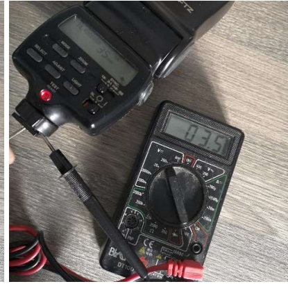
Old Flash but safe trigger voltage.
